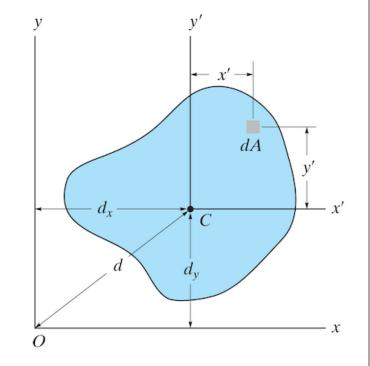
**Note:** the integral over y' gives zero when done through the centroid axis.
