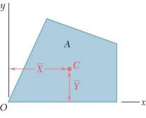
• In the case of a composite area, we divide the area A into parts  $A_1, A_2, A_3 =$
